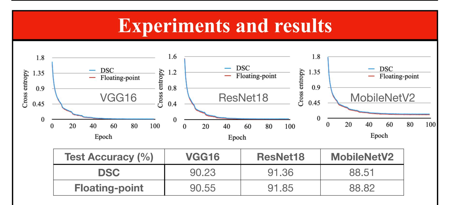
The convergence of cross entropy, test accuracy are compared with the floating-point implementation using the same settings.
